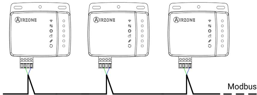
For proper operation of the system, verify that only the communication cables (green-blue) are connected to their matching domotic buses. Attach the wires with the terminal screws following the color code.
