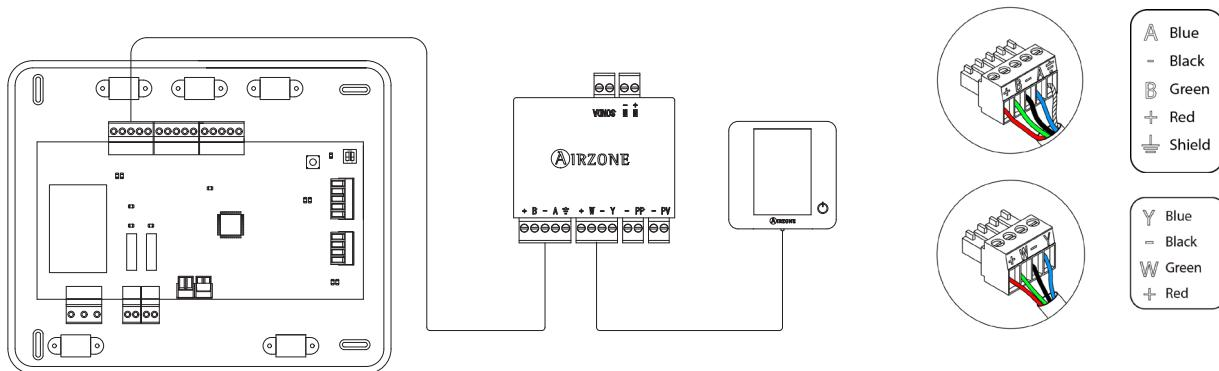
Do not connect the “-” pole to the “+” terminal. It may damage the device.
