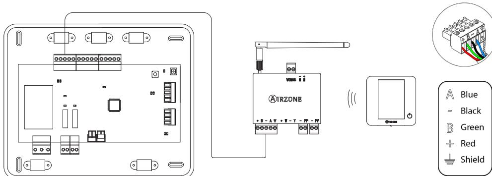
Do not connect the “-” pole to the “+” terminal. It may damage the device.
