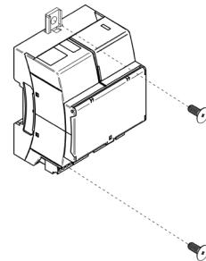
**Note:** To remove the module on DIN rail, pull the tab downwards to release it.
