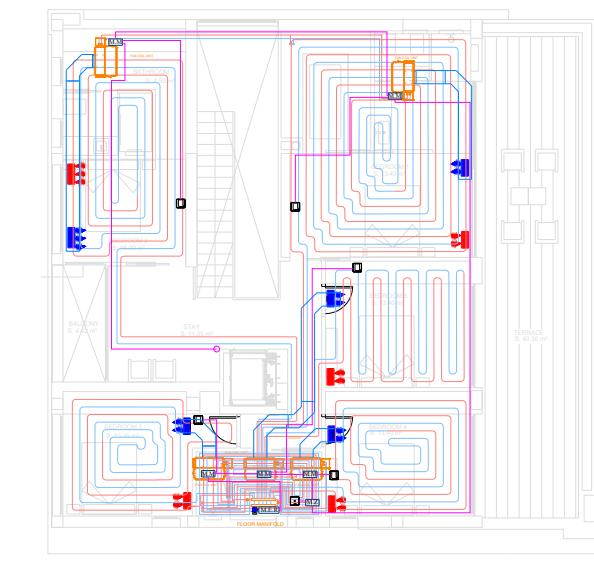
The layout of the villa is shown in the above plans, using individual fan coil units and an underfloor heating and cooling system with an air to water heat pump, secondary pumps and a dual set-point (cooling/heating) mixing valve.
