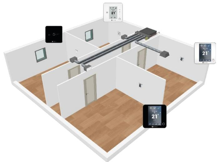
Figure 1. Diagram of a zoned system
