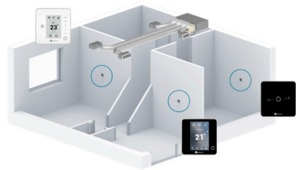
Figure 1. Diagram of a zoned system.
