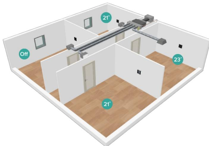
An Airzone Integrated Zoning System transforms a traditional ducted HVAC system into a multizone system, basing its operation on two main factors:
